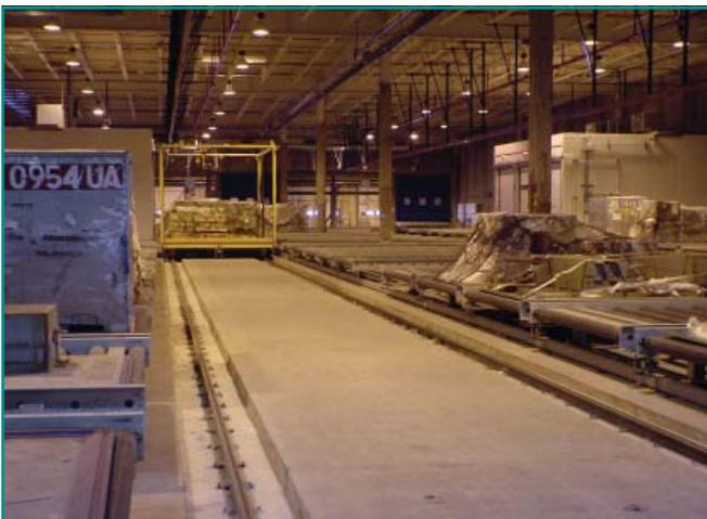
The containers, which might weigh as much as 30,000 lbs., are moved horizontally along rollers or vertically on lifts. PROVOTON foam concrete will provide a settlement free backfill for United's automated cargo handling track system.
